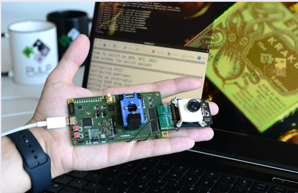
Fig.7: Application board using the Kraken chip connected to an event-based camera system.
